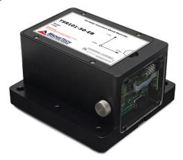
The TSR101-EB is a battery powered, stand alone transient tri-axial shock recorder. The TSR101-EB measures and records instantaneous shock levels when the user-selectable shock levels have been exceeded. There are 15 rates to chose from ranging from 1024Hz to 1 Hz. The TSR101-EB is valuable in characterizing environments such as railcar coupling impacts and aircraft turbulence monitoring.
